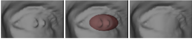
Figure 6: Regionally constrained smoothing. Left: Laser scan reconstruction with unwanted, pointed artifacts in the eye. Middle: Defining the region to be smoothed with a (red) superellipsoid. Right: Smoothing the surface within the superellipsoid. The surface is constrained to only move inwards.
